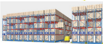
Mobile Rack for the requirement of higher storage capacity Total storage area = 550 m 2 Pallet locations = 1,500 Pallets
