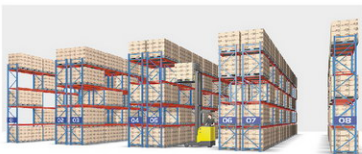
Selective Rack in conventional arrangement Total storage area = 550 m 2 Pallet locations = 800 Pallets
